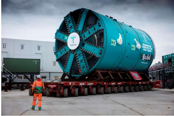
TBM Rachel – 7 metres in diameter
